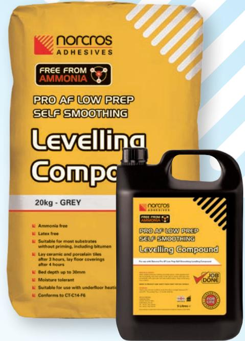
Pro AF 2-Part Low Prep Self Smoothing Levelling Compound is suitable for use on most substrates without the need for priming. It is particularly suitable for use over old adhesive residues and bitumen due to its low compressive strength. A bed depth of up to 30mm can be achieved with the addition of 3mm single-size granite chippings.
